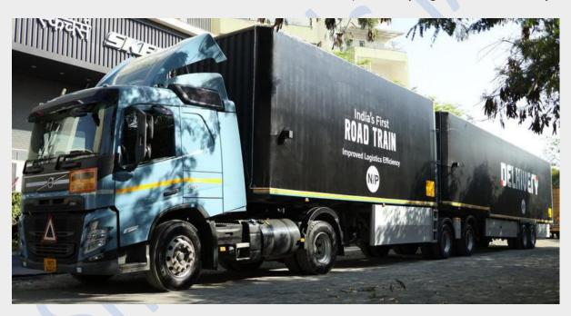
The concept was formally incorporated into regulations in 2020, allowing for vehicle lengths of up to 25.25 metre. A road train consists of a tractor unit towing two or more trailers.
