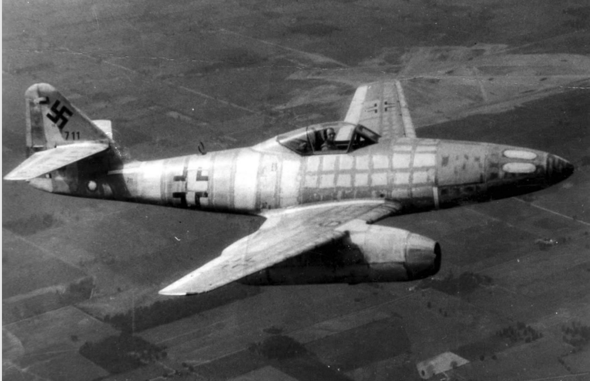
The Messerschmitt Me 262 Schwalbe, developed by Germany during World War II, is considered to be the world's first jet fighter. (USAF)
